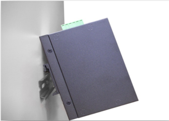
Figure 3.2 - Insert the Switch on the DIN-Rail
